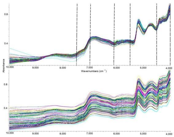
**Figure 2:** Sample universe with an averages spectra of 100 species (332 samples) of wood from the Amazonian region in the range of 10,000-4,000 cm<sup>-1</sup>. At the bottom are raw spectra, and at the top are pre-processed spectra with multiplicative scatter correction (MSC) with Savitzky-Golay filters.
