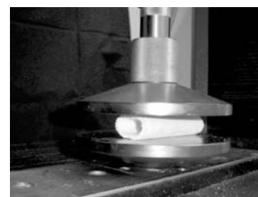
Figure 7 – Compression assay (cylinders).
