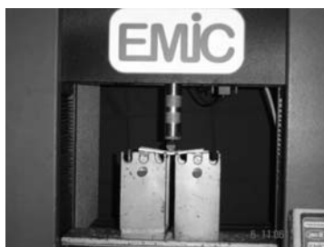
Figure 6 – Flexion assay on 3 points (plates).
