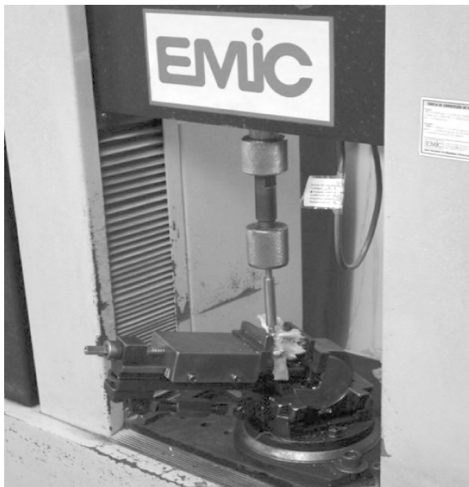
Figure 1 - Universal assay machine for testing pedicular screws' pullout strength.
