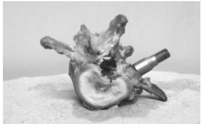
Figure 2B - Vertebra after screw's pullout test. Here, we can notice the cortical rupture.
