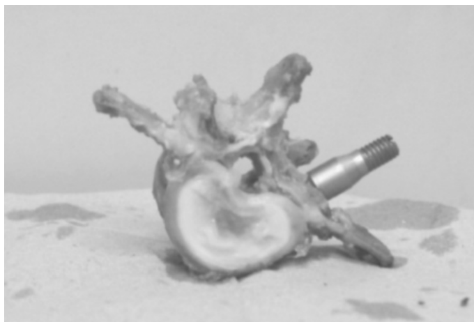
Figure 2A - Vertebra with pedicular screw before the pullout test.
