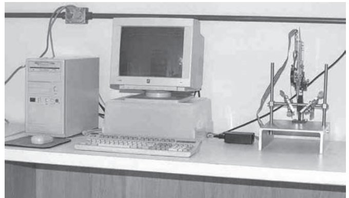
Figure 2 – Computerized equipment for weight drop impact - Impactor.
