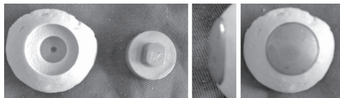
Figure 2 – The cupuliform patellar implant, fitted into a milled circular recess, with a depth of 5mm, with a groove at the center for a 5mm deep fixation pin.
