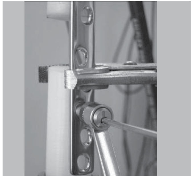
Figure 4. Assembly for execution of eccentric hole, with guide and drill bit, both from the same manufacturer as the tested plate.
