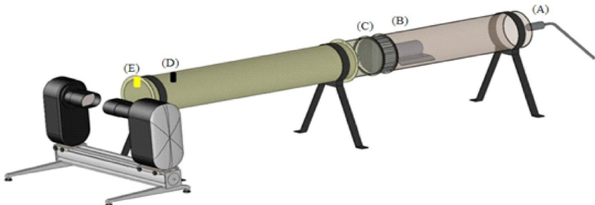
Figure 1. Prototype used in the experiment: Gas heater (A), Fan (B), Air homogenizer (C), Sensors of temperature and relative air humidity (D) and Hydraulic nozzle (E)
