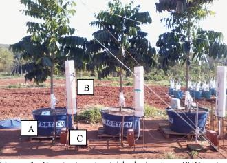
Figure 1. Constant water table lysimeters: PVC water tank (500-L capacity) (A), PVC water reservoir (pipe with diameter of 200 mm and height of 1.50 m) (B) and discharge box (C)
