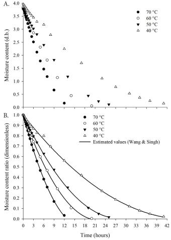
Figure 1. Experimental moisture content (A) and moisture content ratio (B) of 'okara' (decimal, d.b.) with values obtained experimentally and estimated by the Wang & Singh model, as a function of drying time (hours) for the temperatures of 40, 50, 60 and 70  $^{\circ}$ C
