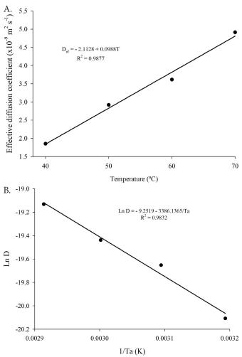
Figure 2. Mean values of the diffusion coefficient ( $m^2 s^{-1}$ ) obtained for 'okara' drying (A) and Arrhenius representation for the diffusion coefficient as a function of drying air temperature (B)
