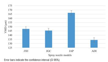
**Figure 2.** Volumetric mean diameter (VMD) of the spray nozzles with inclined flat jet (J3D), inclined flat jet with pre-orifice (JGC), second-generation air-induction inclined flat jet (JAP) and flat jet with pre-orifice (ADI)
