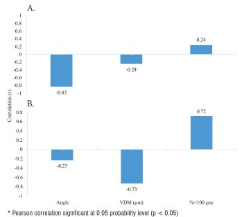
**Figure 4.** Correlation between collected drift with jet angle, VMD and  $\% < 100 \ \mu$ m. (A) Against wind flow direction (upwind); (B) Along wind flow direction (downwind)
