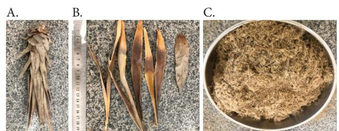
**Figure 1.** Fibers used: raw pineapple crown (A); separation of crown parts (B); fibers in their final form, before heat treatment (C)
