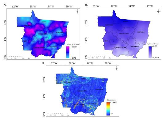
Figure 2. Maps of (A) rainfall erosivity, R, (B) soil erodibility, K, and (C) the topographic factor, LS, for the state of Mato Grosso, Brazil
