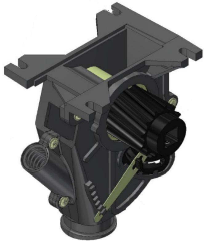
**Figure 1.** Constant flow seed metering device with helicoidal fluted roller
