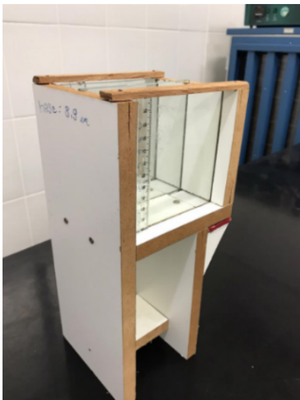
Figure 2. Prototype used to determine the angle of repose
