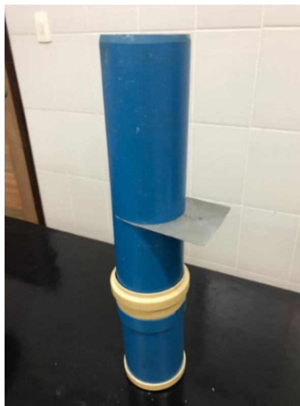
Figure 1. Prototype used to determine the bulk density of cowpea grain samples
