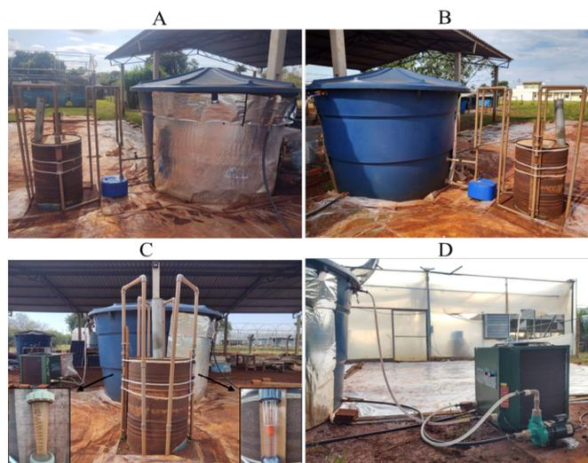
**Figure 3.** Circuit for the passage of water in (A) PVC pipe and (B) copper pipe, (C) Rotameters and (D) Water heating system
