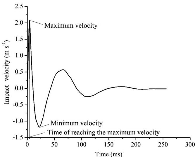
**Figure 2.** Velocity curve of the potato during impact
