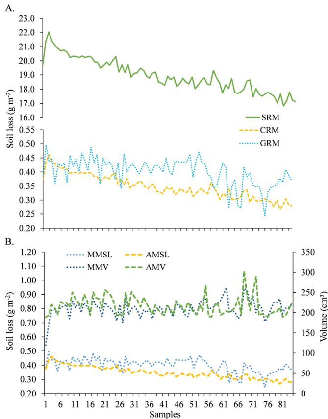
SRM - Simulated runoff method; CRM - Collected runoff method; GRM - Gravimetric method; MMSL - Manually measured soil loss; AMSL - Automatically measured soil loss; MMV - Manually measured volume; AMV - Automatically measured volume
