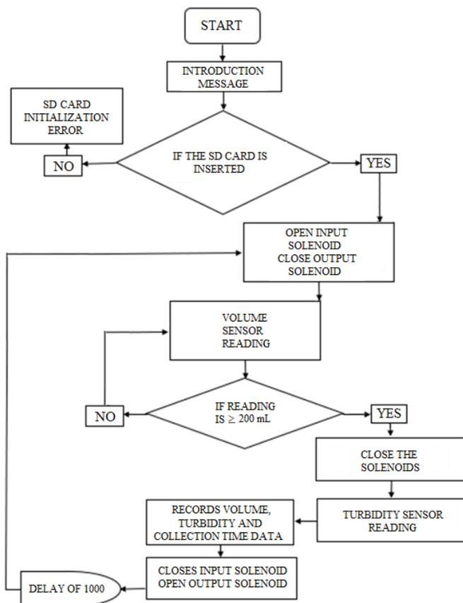
**Figure 3.** Flowchart of the programming used in the prototype of the runoff collector for readings made using a pre-defined volume of 200 cm<sup>3</sup>
