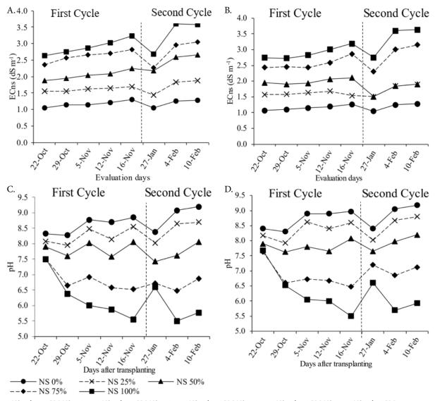
NS 0% - 0% NS and 100% RW; NS 25% - 25% NS and 75% RW; NS 50% - 50% NS and 50% RW; NS 75% - 75% NS and 25% RW; NS - 100% NS and 0% RW **Figure 2.** Electrical conductivity of the nutrient solution (EC<sub>ns</sub>) and pH values observed during first (A and C) and second (B and D) production cycles for different recirculation times - T1 (A and C) and T2 (B and D)
