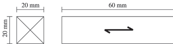
Figure 1. Dimensions of the test specimens.
