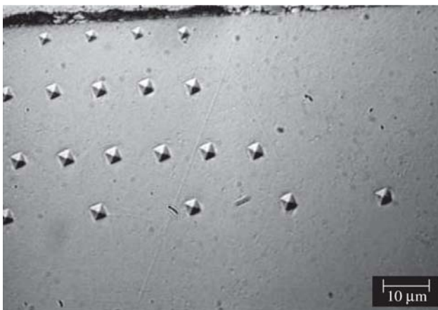
Figure 8. Vickers impressions taken beneath the nitrided layer of a H13 tool steel specimen. Load = 50 mN.
