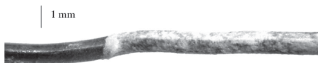
Figure 1. Image of the platinum electrode surface covered with the organic film after 90 minutes of anodic growth with the application of 10 mA of current, taken with a digital camera with zoom.
