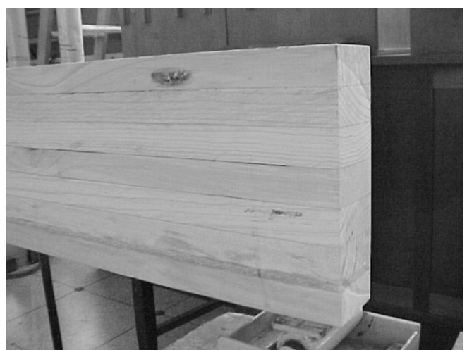
Detail of the reinforced beam.
