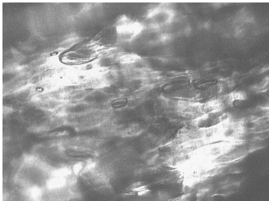
Figure 1. Birefringence observed in liquid crystals formed from Renex-100™.
