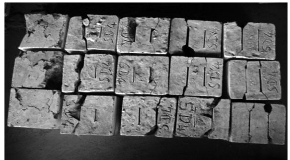
Cubes DCN - a/w = 0.3 DCN - a/w = 0.4 DCN - a/w = 0.5 DCN - a/w = 0.6 Crack patterns after testing with 100% replacement of natural sand with crushed stone fine aggregate (e)
