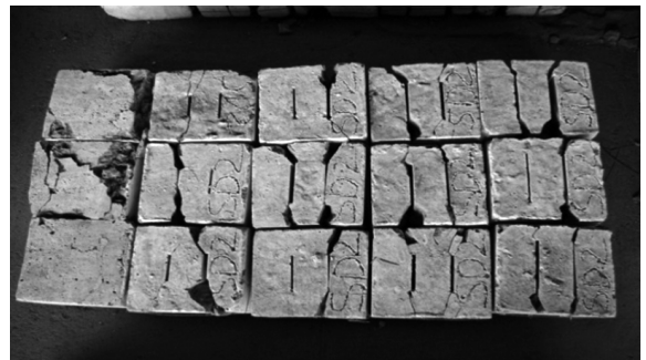
Cubes DCN - a/w = 0.3 DCN - a/w = 0.4 DCN - a/w = 0.5 DCN - a/w = 0.6 Crack patterns after testing with 50% replacement of natural sand with crushed stone fine aggregate (c)
