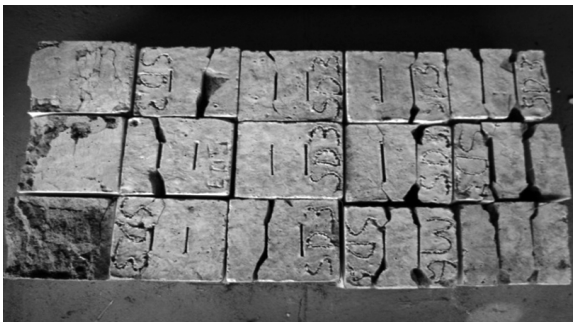
Cubes DCN - a/w = 0.3 DCN - a/w = 0.4 DCN - a/w = 0.5 DCN - a/w = 0.6 Crack patterns after testing with 75% replacement of natural sand with crushed stone fine aggregate (d)
