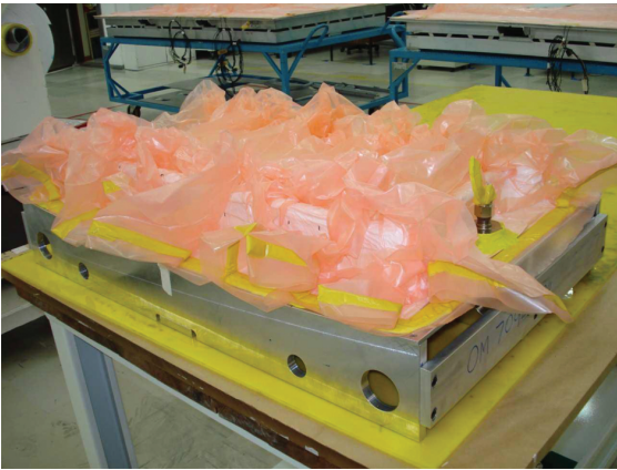
Figure 3. Vacuum bag assembling, just before the autoclave forming.
