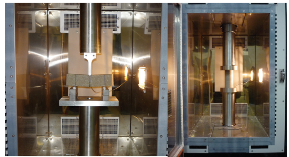
Figure 2. Flexural and compressive test set-up in the Universal Testing Machine.
