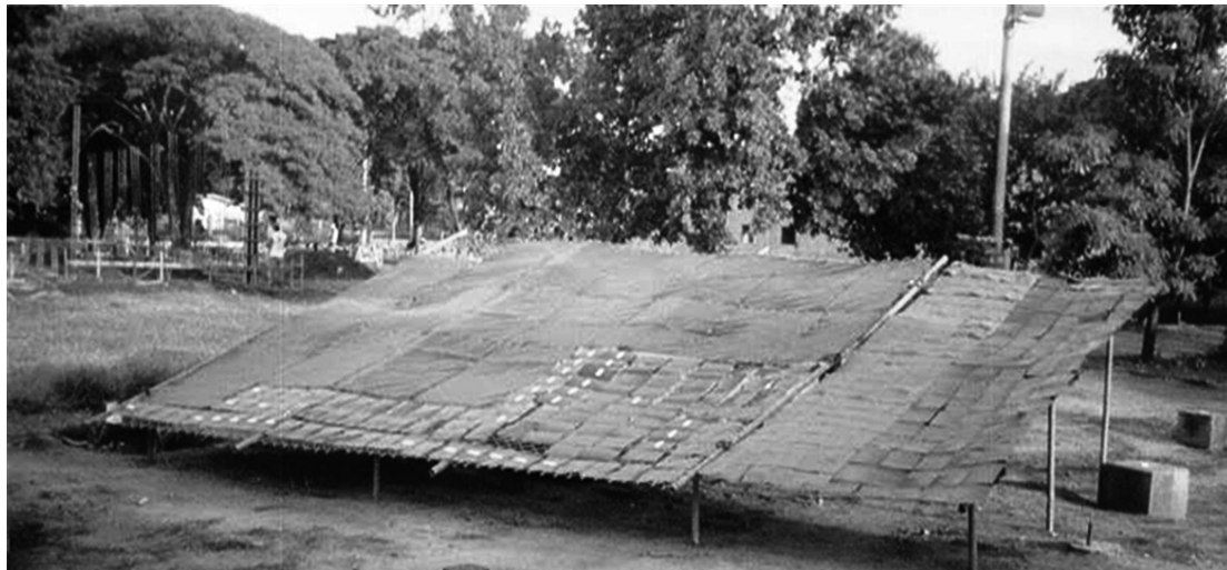
Figure 1. HDPE and PVC geomembranes samples exposed to weathering.
