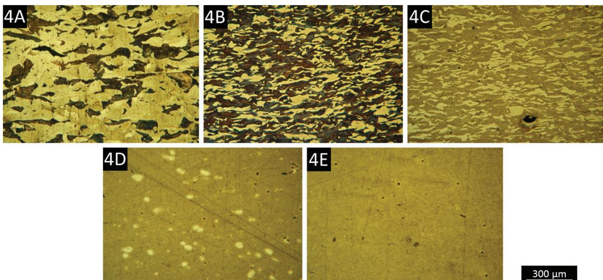
**Figure 4.** Microstructures of the hot pressed sterling silver processed at a pressure of 35MPa for 60 minutes at different temperatures: A) 250 °C; B) 300 °C; C) 400 °C; D) 500 °C and E) 700 °C.
