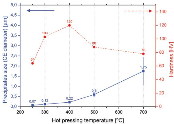
**Figure 9.** Plot of the relationship existing between the size of the Cu-rich precipitates ( $\beta$  phase) and the hardness measured in hot pressed sterling-silver compacts (Ag-Cu alloy) at a pressure of 35MPa for 30min and at different temperatures. CE = Equivalent Circular Diameter.
