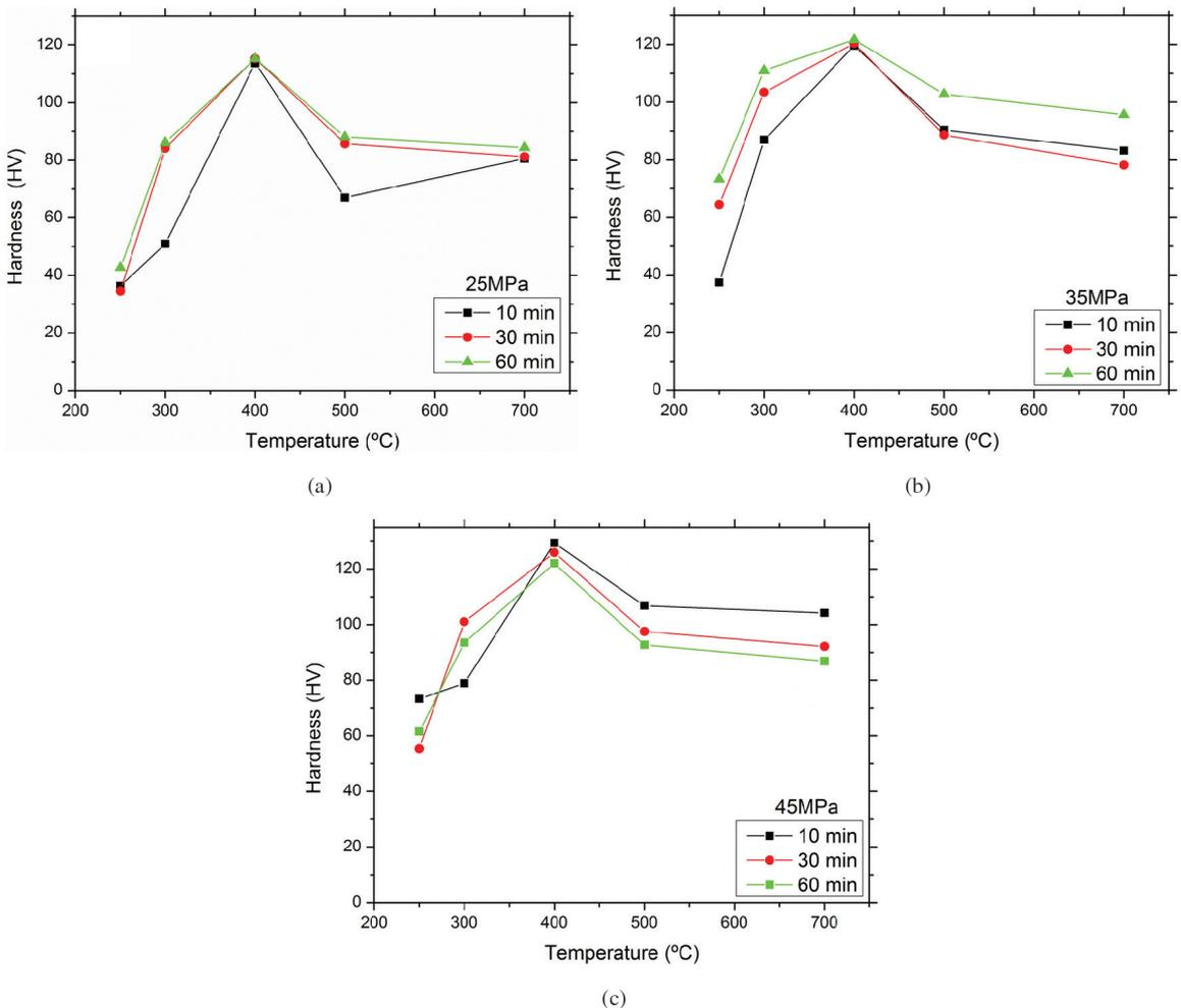
**Figure 8.** Influence of the processing parameters (pressure, time and temperature) on the hardness of the hot pressed sterling silver powder compacts.
