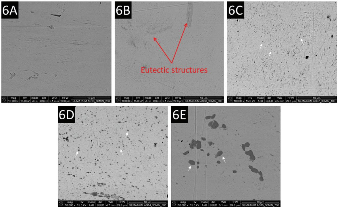
**Figure 6.** SEM micrographs of hot pressed sterling silver compacts processed at a pressure of 35MPa for 30min at different temperatures: A) 250 °C; B) 300 °C; C) 400 °C; D) 500 °C and E) 700 °C. White arrows indicate the Cu-rich precipitates ( $\beta$  phase).
