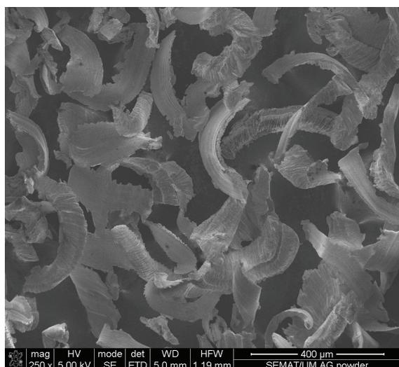
Figure 1. SEM micrograph showing the morphology of the silver alloy powders.
