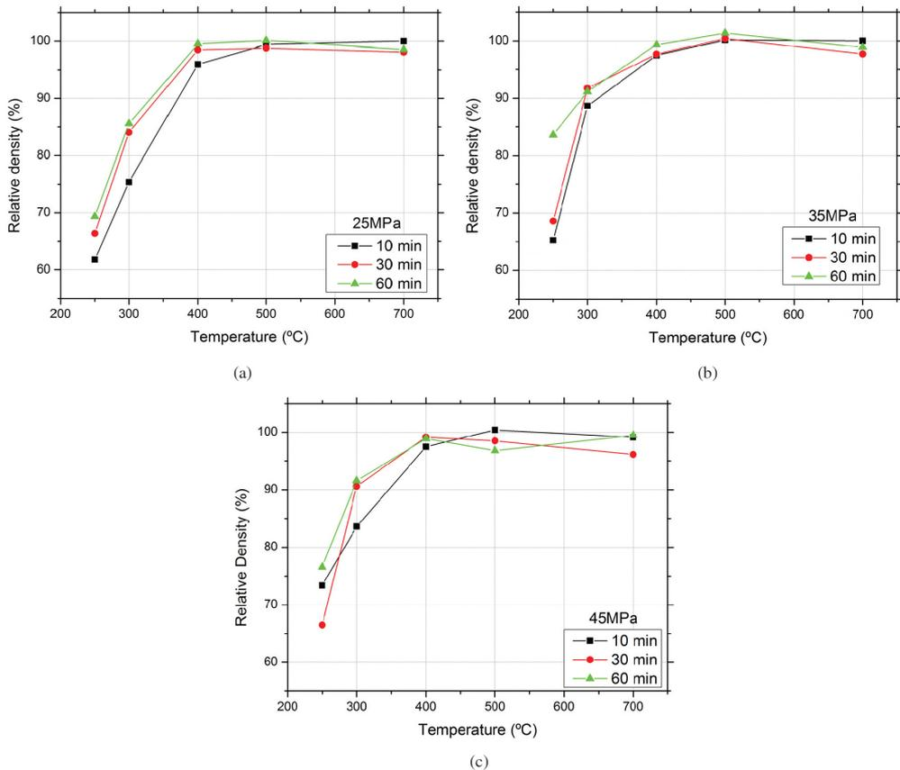
**Figure 7.** Influence of the processing parameters (pressure, time and temperature) on the relative density of the hot pressed sterling silver powder compacts.
