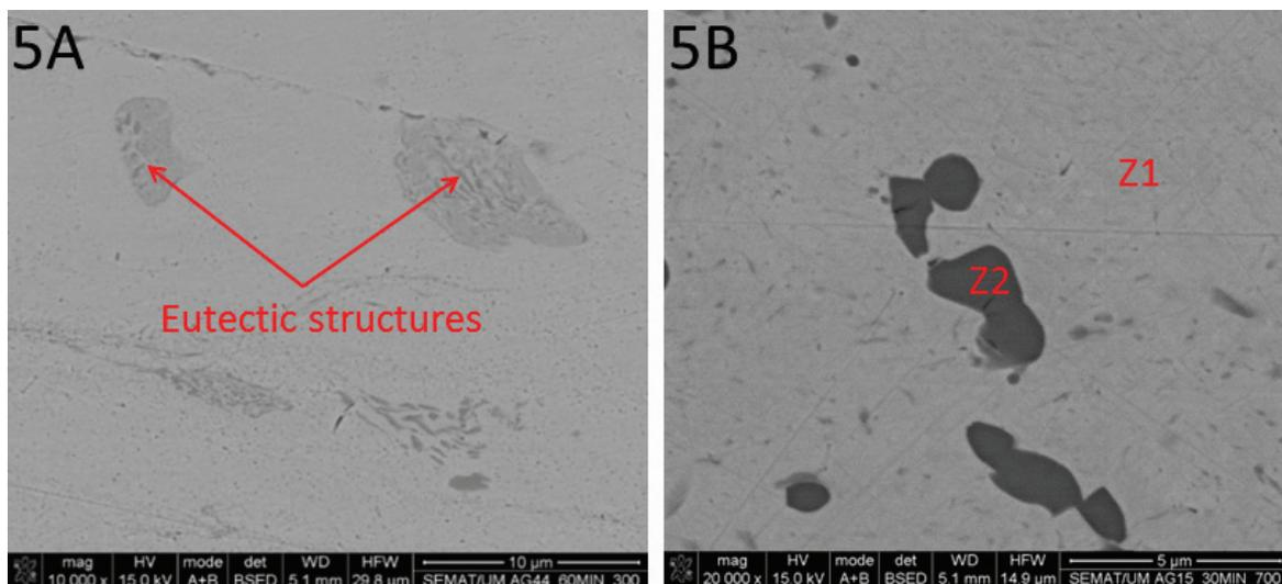
**Figure 5.** Micrographs of the hot pressed sterling silver compacts. A) 300 °C, 60min, 35MPa; B) 700 °C, 30min, 35MPa. The dark phase refers to a Cu-rich phase ( $\beta$  phase).
