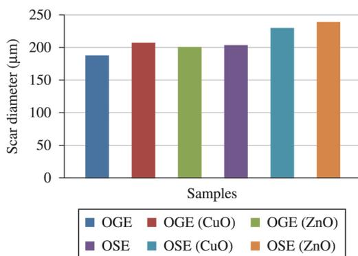
**Figure 3.** Wear Sphere observed in lubricants analyzed. OSE (epoxidized soybean oil); OSE (CuO) (epoxidized soybean oil with Copper Oxide Nanoparticle); OSE (ZnO) (epoxidized soybean oil with Zinc Oxide Nanoparticle); OGE (Sunflower Oil Epoxidized); OGE (CuO) (Sunflower Oil with Copper Oxide Nanoparticles); OGE (ZnO) (Sunflower Oil Epoxidized with Nanoparticles of Zinc Oxide).
