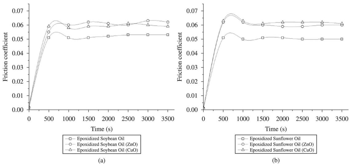
Figure 1. Coefficient of friction behavior for biolubricants: a) epoxidized soybean oil and b) epoxidized sunflower oil.
