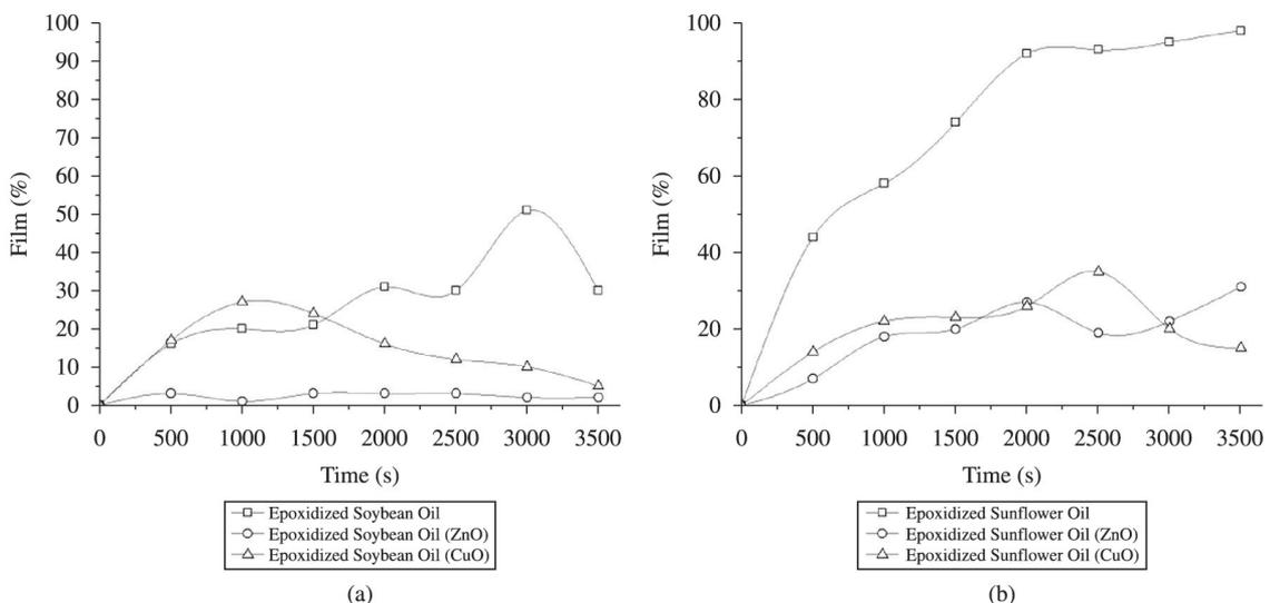
Figure 2. Film formation behavior for biolubricants: a) epoxidized soybean oil and b) epoxidized sunflower oil.
