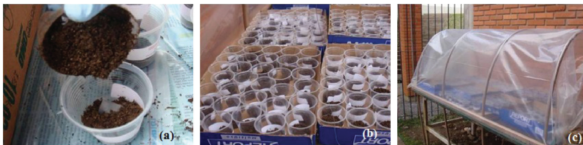
Figure 2. Exposure of samples in (a) cups with the simulated soil and the polymeric samples, (b) greenhouse dispose and (c) greenhouse.
