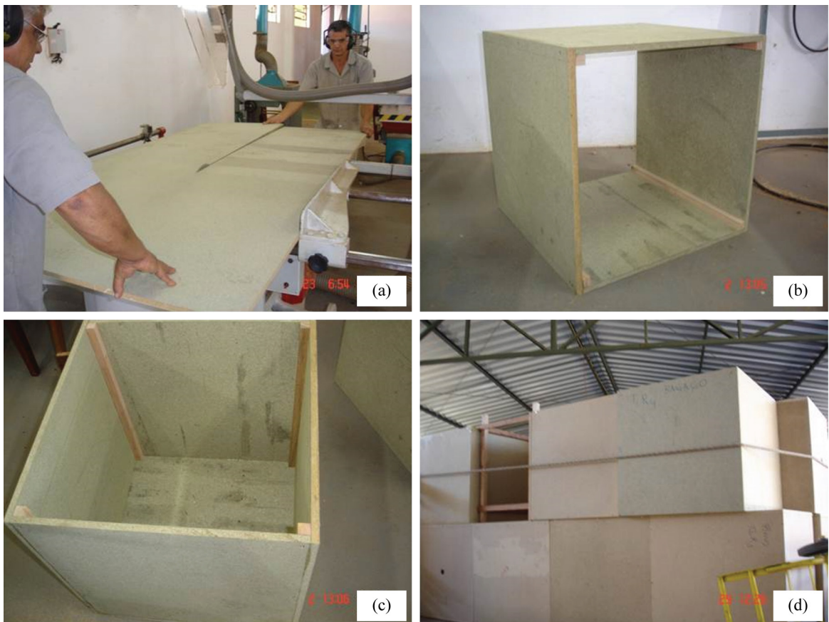
Figure 1. Development of modules; (a) Acquired panel; (b) and (c) Module assembly; (d) Set of modules tested.
