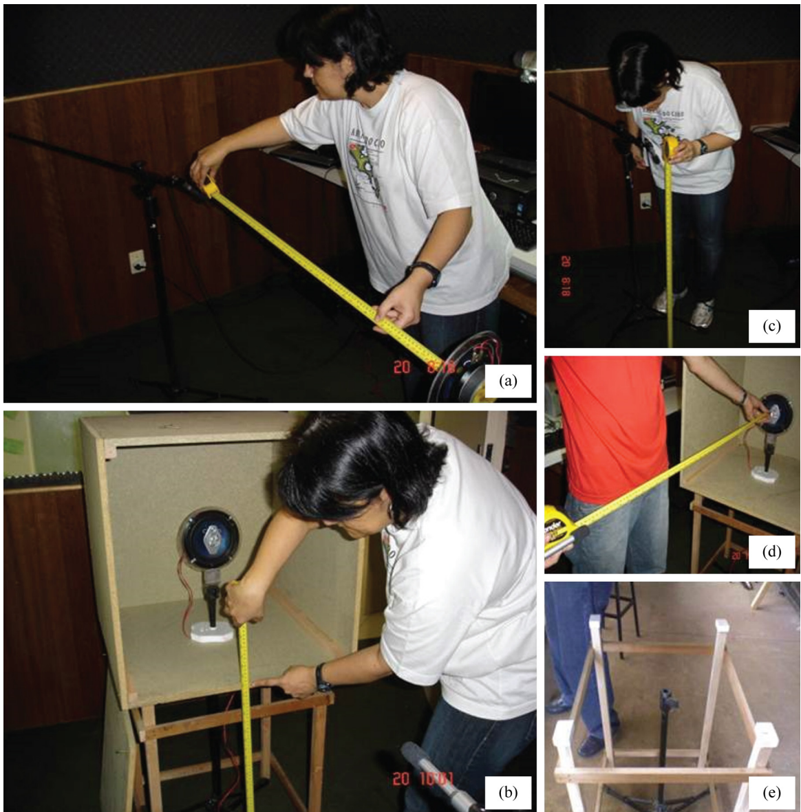
Figure 4. Photos of the assembly of the experiment; (a) Positioning for characterization of the source of noise; (b), (c) and (d) Positioning with the modules and (e) Rubber buffer supports.
