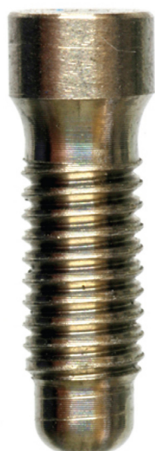
Figure 2. Ti implant with macrostructure of rounded tip and apex profile equal to Zr implant.
