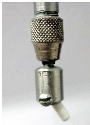
Figure 3. Device to insert implants coupled to the parallelometer used to insert implants in polyurethane resin at an angle of 30°.
