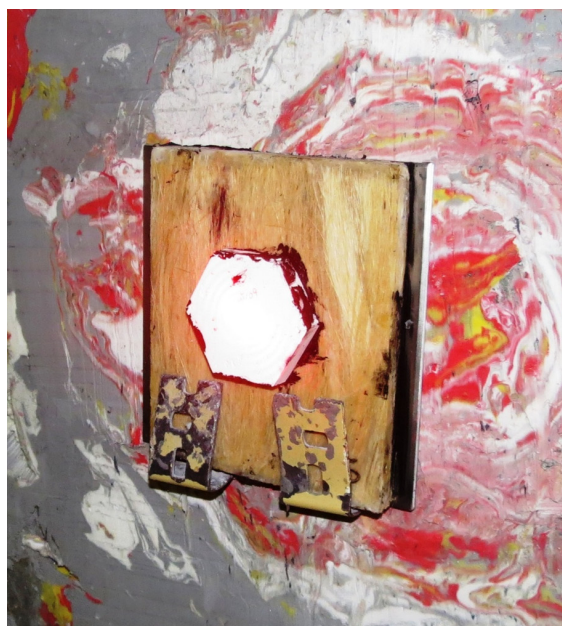
Figure 2. Complete multilayered armor clamped into the clay witness and ready to be ballistic tested.
