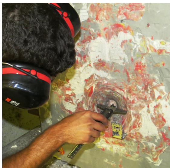
Figure 3. Measurement of the indentation in the clay witness caused by the projectile impact.
