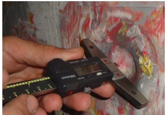
Figure 3. Measurement of the depth of penetration in the clay witness caused by the projectile impact.
