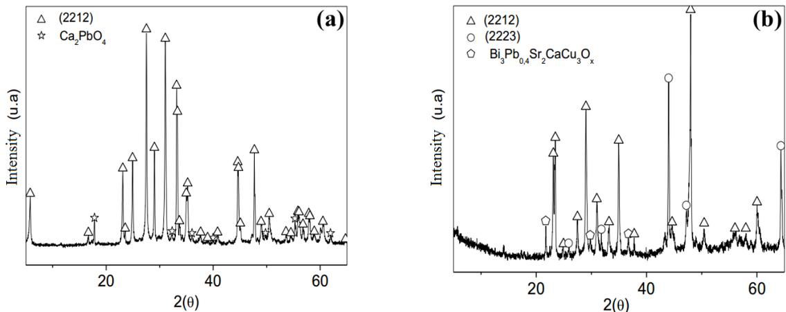
Figure 2: X-ray patterns of BSCCO powder: (a) treated sample (film) by using microwave-oven (b) commercial powder.
