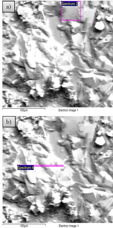
**Figure 4:** EDS analysis of the different structures presented by the treated sample (a) Smooth and (b) Roughness area.
