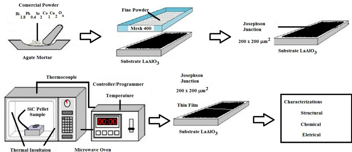
Figure 1: Experimental scheme for the sample preparation [9].
