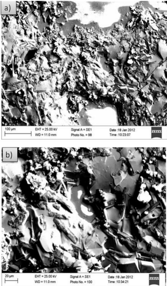
**Figure 3:** SEM images for the junction built in the BSCCO film: (a) Junction view, and (b) detailed of the structure observed at the junction.
