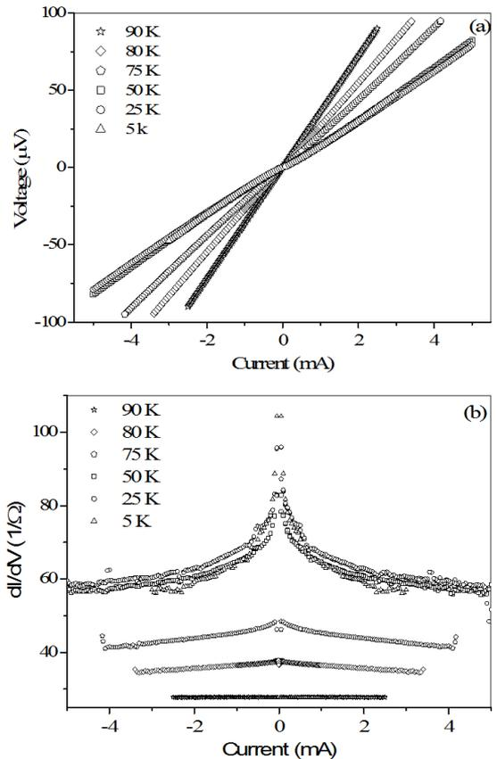
**Figure 6:** Characteristic curves as function of temperature: (a) Voltage versus electrical current ( $V \times I$ ), and (b) Derivative curve  $dI/dV$  versus electrical current ( $I$ ).
