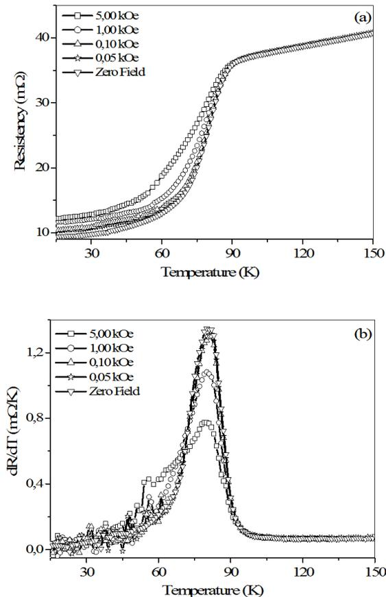
**Figure 5:** Electrical characterization of the sample to different values of electrical current applied: (a) Electrical resistance versus Temperature, and (b) Derivative curve  $dR/dT$  versus  $T$ .
