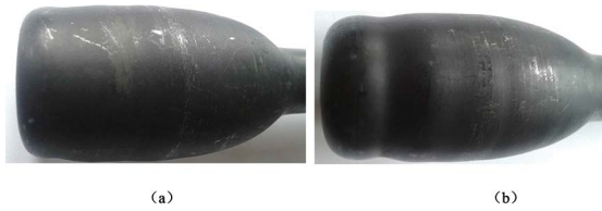
Figure 13: The forming results in experiment (a) under the three-stage current mode, (b) under the constant current mode.
