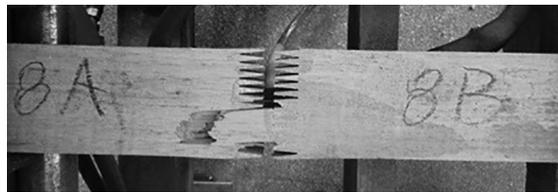
**Figure 5:** Specimen with finger joint right after rupture (50% in the wood and 50% in the glue).
