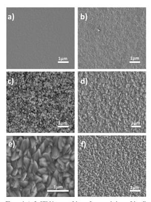
**Figure 1:** (a-f). SEM images of the surface morphology of the all samples. a and b) Samples A and B, c-f) Doped samples (SnO<sub>2</sub>:F) synthetized at different temperature and deposition time
