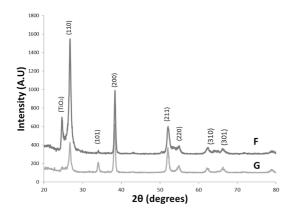
**Figure 3:** GIXRD patterns of doped samples with fluorine. (Samples F and G). These samples presented only single-phase cassiterite structure.
