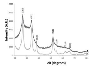
Figure 2: GIXRD patterns of SnO<sub>2</sub> samples (A and B).
