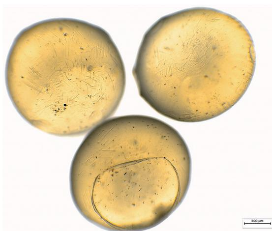
**Figure 5:** Images obtained by optical microscopy of dried alginate microparticles at 3% alginate +  $0.1 \text{ mol.L}^{-1} \text{ CaCl}_2$  + NaCl.
