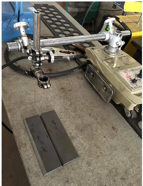
Figure 3. Gas-cutting machine.
