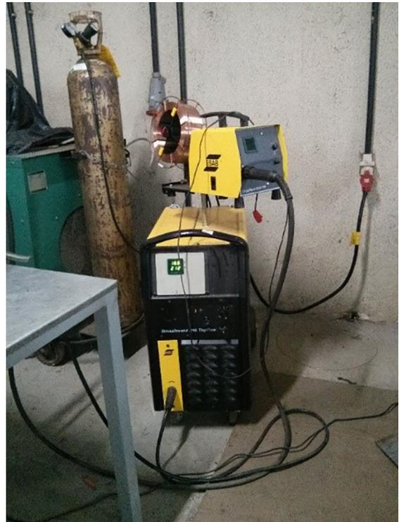
Figure 2. MAG welding semiautomatic machine.
