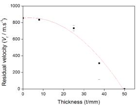
Figure 2. Residual velocity of the bullet after impact against the targets as a function of the laminate thickness.
