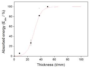
Figure 3. Fraction of the bullet's energy absorbed by the laminates, as a function of thickness.
