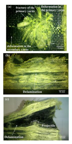
**Figure 5.** Damage inflicted to the aramid laminates: (a) 48 layers, perforation hole; (b) 72 layers, cross-sectional area; and (c) 96 layers, cross-sectional area.
