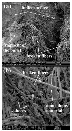
**Figure 6.** SEM micrographs of the bullet's surface after the impact: (a) 100x; (b) 500x.
