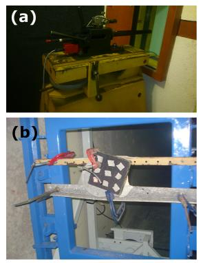
Figure 1. Experimental arrangement of the ballistic tests: (a) gun barrel with laser sight; (b) aramid sample mounted as target.
