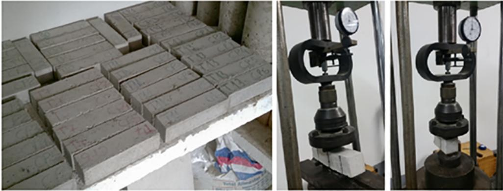
Figure 1. Flexural and compressive strength tests with (4 x 4 x 16) cm prism specimens.
