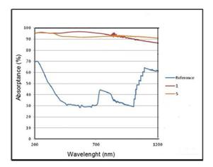
Figure 5. Spectroscopy of the substrate and the samples 1 and 5 coated.
