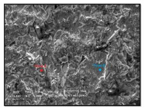
Figure 3. Microstructure of the sample 1 coated with black chromium.
