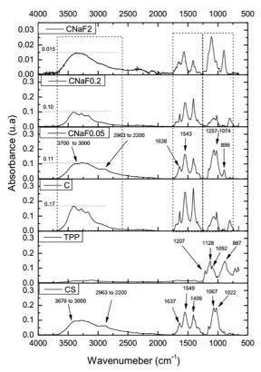
Figure 1. FTIR spectra of: TPP, Chitosan Solution (CS), Chitosan Particles (C), CNaF0.05, CNaF0.2 and CNaF2, respectively for 0.05%, 0.02% and 2% NaF.
