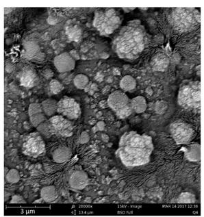
Figure 3. Particles micrographs / EDS CNaF2 20.000X.
