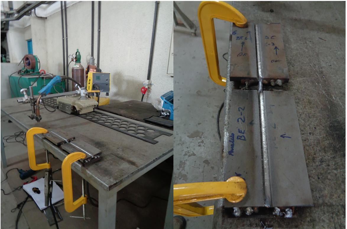
Figure 2. Apparatus mounted for welding
