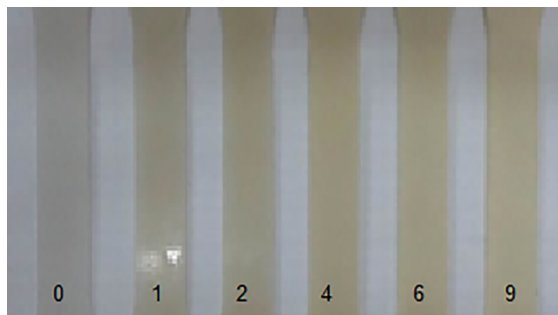
Figure 1. Photographs of PCL specimens illustrating light-yellowing after UV-B exposure. Exposing times in weeks are indicated
