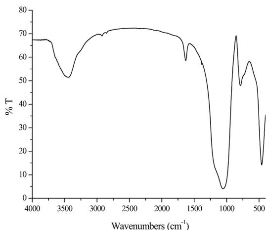
**Figure 4.** Transmission FT-IR/MIR Spectrum of neat PExp, prepared as KBr pellets (0.8:400 mg KBr).
