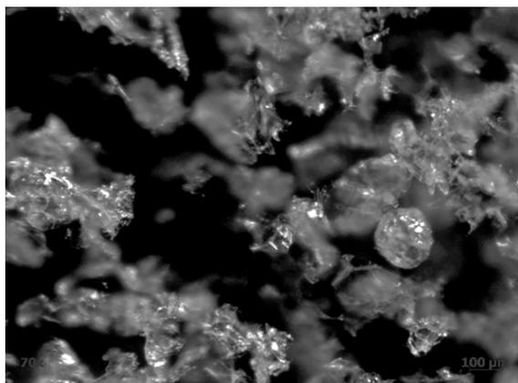
**Figure 3.** Stereomicrography of neat PExp. Magnification: 70x.
