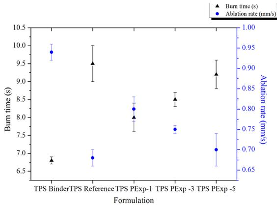
**Figure 9.** Burn time and Ablation rate with an oxyacetylene torch for the formulation studied
