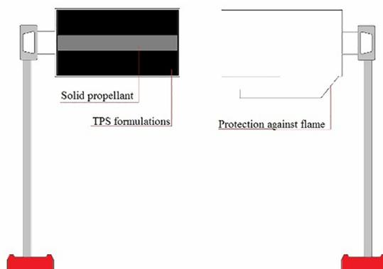
**Figure 2.** Propellant Ablation Test apparatus.
