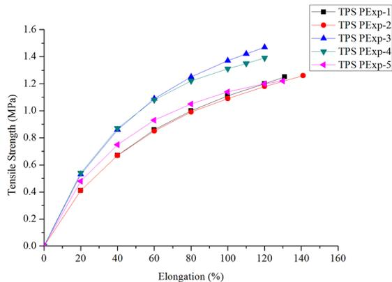
**Figure 7.** Tensile strength versus elongation profile for the TPS PExp samples.
