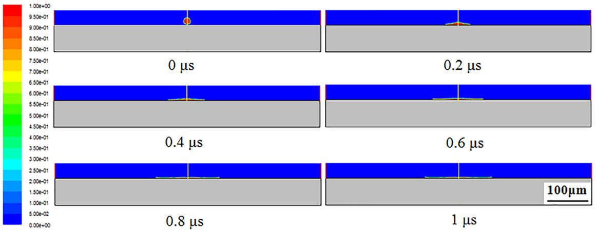
**Figure 2.** Deformation and solidification process of TWAS droplet ( $\phi 25 \mu\text{m}$ , 100 m/s).
