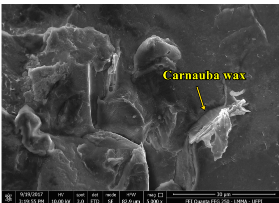
Figure 8. Scanning electron microscopy of the fracture surface of PBAT/SR/CW - 2.5, with a magnification of 5000x. (colored in the online version)
