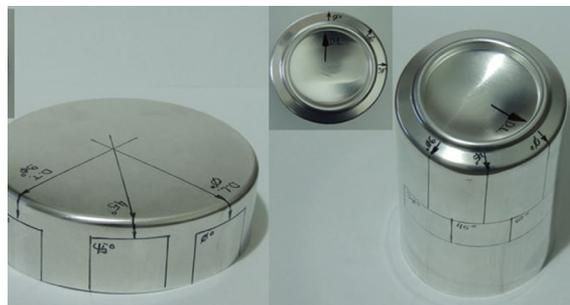
**Figure 2.** The first stage (drawn cup) and last stage (after the 3<sup>rd</sup> ironing die) used in acquiring samples forming the different angles in relation to the rolling direction.
